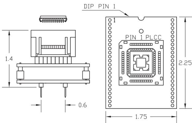
Press rim to open socket, Press device to close
